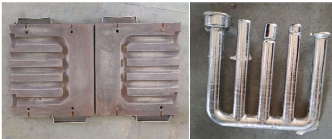
Fig.2 (a) Metallic Die (b) Casting after solidification
